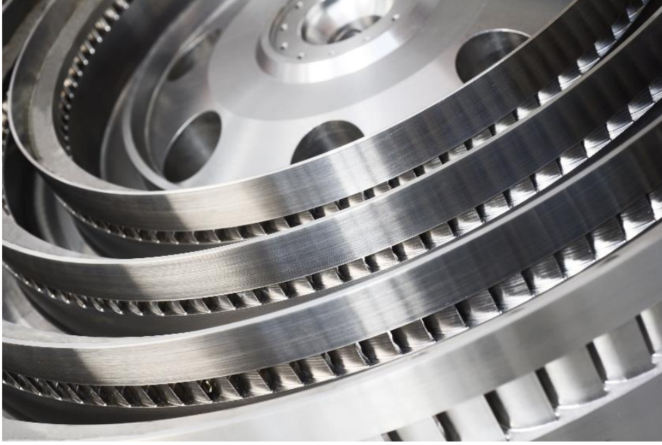
Figure 4. Rotor disk of the Bagnore radial outflow turbine.
