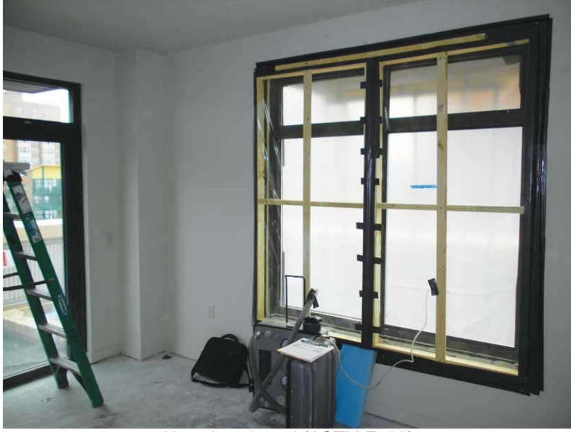
Hava kaçak testi (ASTM E783)
